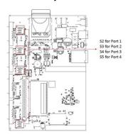
Dip switch Pin 1 and Pin 2 are used to set the pull up/down resistors. The default is 150 K $\Omega$ . Turn on dip switch Pin 1 and Pin 2 to set this value to 1 K $\Omega$ . Do not use the K $\Omega$  setting with RS-232 mode, since doing so will degrade the RS-232 signals and shorten the communication distance. Dip switch Pin 3 is used to set the terminator. Turn on dip switch Pin 3 to set this value to 120 ohm.
