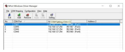
On the **Basic Setting** window, use the **COM Number** drop-down list to select a COM number to be assigned to the NPort 5000's serial port that is being configured. When you have selected multiple ports, you may select the **Auto Enumerating COM Number for Selected Ports** option to automatically assign available COM numbers in sequence to selected serial ports. Note that ports that are "in use" will be labeled accordingly.
