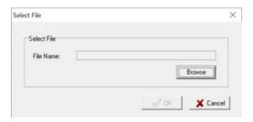
For the overall NPort 5000 Series with security enhanced firmware version, export configuration encryption will be based on the Pre-shared key defined in the NPort (default is empty password, and you may configure the password in **Configuration > Configuration Pre-shared Key**. So, when you are exporting the configuration file, you are only required to select the output file location. You may refer to page 96 for the security firmware version of your NPort.
