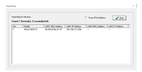
When the search is completed, all NPort 5000 serial device servers that are located are displayed in the DSU window. Select the device you wish to access and press the **Unlock** button to input the username and password for the device.
