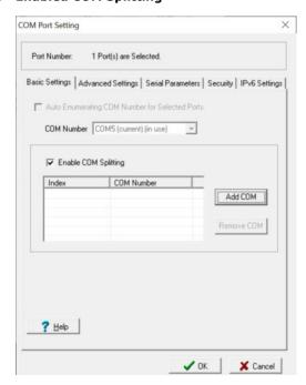
2. Add COM to select target COM ports for splitting; the COM port must be available.
