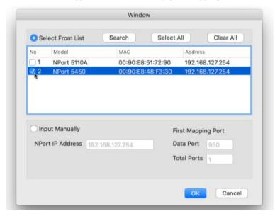
NPortConnect would auto assign the tty name and corresponding port number to the IP address of the selected NPort.
