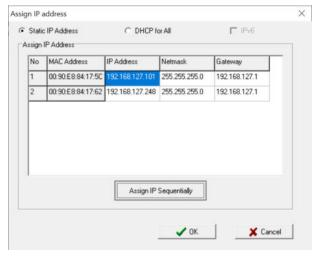
3. Click on the IP Address box to input the IP address manually. Do the same action to the **Netmask** cell as well. If multiple units of the same model are selected, you can click **Assign IP Sequentially** so it will assign IP in sequence, starting from the IP address of the first device.
