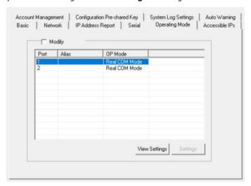
Set the operating mode and associated parameters as needed. Refer to **Chapter 4** and **Chapter 5** for additional information on operating modes and advanced settings. When you are ready to restart the device server with the new settings, click **OK**.
