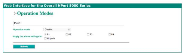
When Operation mode is set to Disabled, that port will be disabled. Select the **Apply the above settings to all serial ports** checkbox to apply this setting to the other ports.
