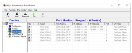
Right-click on Port Monitor and select or deselect **Monitor Items**. Use the single arrowhead buttons to move highlighted items from one box to the other or the double arrowhead buttons to move all items in one box to the other.
