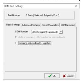
You can view the serial ports that were assigned to and removed from the group. Click Apply to apply the settings.
