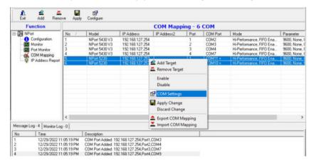
Uncheck Grouping selected port(s) together first then select a COM number for this COM group and check the **Auto enumerating COM number for selected ports** to use the COM number you select as the first starting COM number, and then click **OK**.
