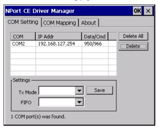
6. To configure the settings for a particular COM port, select the row of the desired port, and then change the setting in the "Settings" panel, as shown below.
