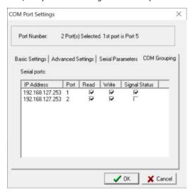
5. Click **OK**, and confirm the serial ports that were assigned. The COM Port column confirms that your selected ports are labeled as part of a "Group." You will be able to view the serial ports that were assigned to and removed from the Group. Click **Apply** to apply the settings.
