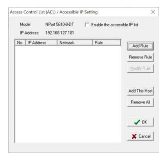
**Enable the accessible IP list:** Turn on or off the Accessible IP function.
