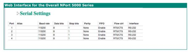
To change serial settings for a particular port, click on the **Port Number** under **Serial Settings**, located under **Main Menu** on the left side of the browser window.
