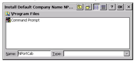
3. Driver installation is now complete and the "NPortCab.cab" icon disappears from the screen. This is normal when installing drivers in Windows CE.
