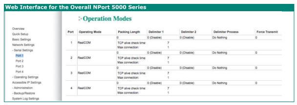
For each mode, the default settings should work for most applications. Change these settings only if necessary for your application. The operation mode and related parameters can be configured through the web console. The same parameters can also be configured using NPort Administrator, the Telnet console, or serial console. Refer to **Chapters 4 and 5** for details.
