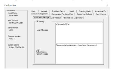
The message will appear on the logn page at the time of a successful login or login failure. Examples are below.
