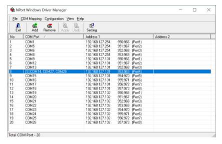
Adjust Max Connection number in the NPort's Operating Settings to match the unit's number in the COM Split Group
