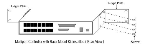
Now the installation of the external Basic/Extensive module is complete. Continue to install the software driver explained in chapter 3.
