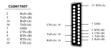
The DTR, DSR and DCD signal lines (not shown) of the C32061T/C32065T are internally shorted by design to meet certain software requirements.
