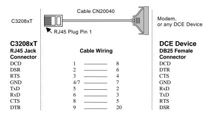
Type 2: Connecting Basic/Extensive Module to a DCE device.
