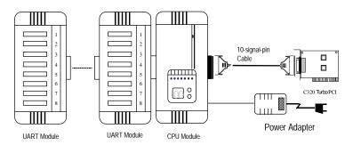
C: Plug the other DB25 female end into the CPU Module's DB25 connector.
