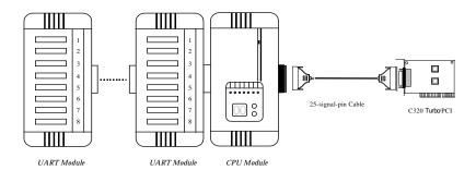
C: Plug the other DB25 female end into the CPU Module's DB25 connector.
