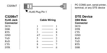
4/7 means either line 4 or line 7 can be used for GND.
