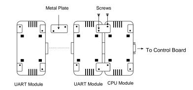
For better fixation of modules, **Fixing Kit** is available and see the bottom view of modules below to install.
