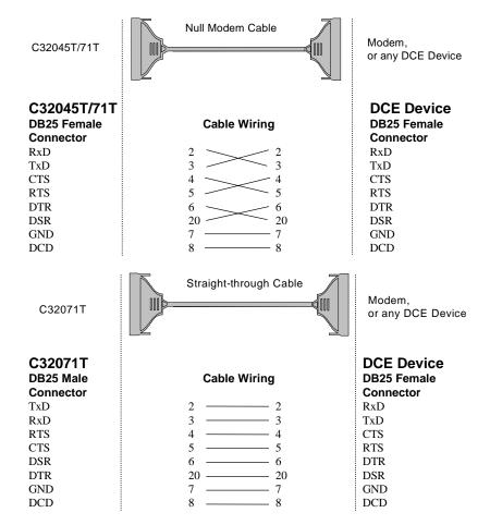
Type 2: Connecting UART Module to a DCE device.
