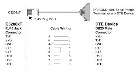
3 4/7 means either line 4 or line 7 can be used for GND.
