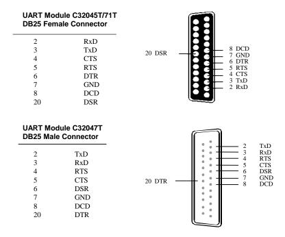
Type 1: Connecting UART Module to a DTE device.
