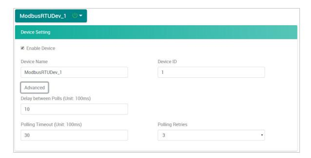
**Device Drop-Down List:** It shows the device name of the Modbus RTU devices. Select one of the devices to configure its settings. The green icon shows that data collection from the device is enabled.
