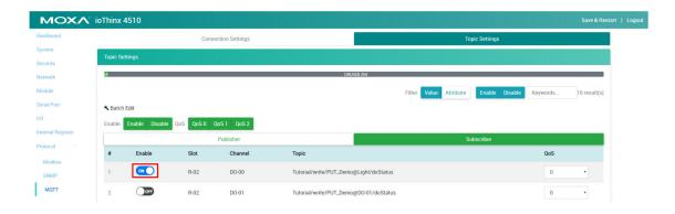
NOTE The content of the **Topic** is based on **Device Name**, **Module name**, and **I/O channel**. You can change these values in **Device Settings**, **Module Settings**, and **I/O Settings**.
