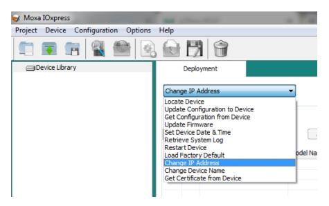
**Step 2:** Select the device(s), change the IP address, type the **username** and **password**, and then click **Submit**. IOxpress will start to execute the task on the selected devices. A message indicating success will appear in the **Result** column if the process was completed successfully.
