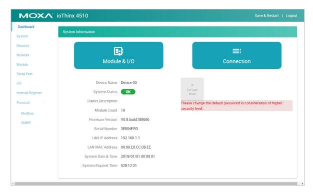
**Exit Safe Mode:** Manually exit the safe mode status of this device. Refer to the **Security** section for more information about the Safe Mode function.
