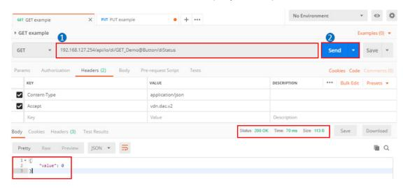
3. Press the DIO button on the starter kit to trigger the DI-00 channel, and then click **Send** again. In response, the DI value will change.
