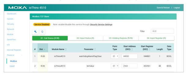
To change Modbus addresses, you can click **Reload default Modbus address**, **Reload current device address**, or manually modify the addresses.
