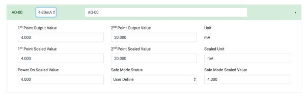
**1st Point Output Value:** The 1<sup>st</sup> point value in the range of channel mode to be scaled to the **1st Point Scaled Value** (range: 0-20 mA mode: 0.000 to 20.000, 4-20 mA mode: 4.000 to 20.000, 0-10V mode: 0.000 to 10.000).
