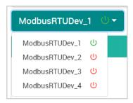
**Enable Device:** Click the checkbox to enable data collection from the device. The icon beside the Modbus device in the **Device Drop-Down List** will change from red to green after being enabled.
