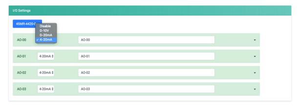
**Channel Mode Drop-down List:** It lists all of the channel modes which can be operated by this channel. Select **Disable**, **0-10 V**, **0-20 mA**, or **4-20 mA** for each channel.
