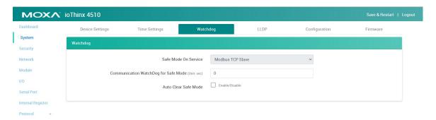
**Safe Mode on Service:** Select the service that you want to link the watchdog to in order to keep monitoring the connection status (option: Modbus TCP Slave).
