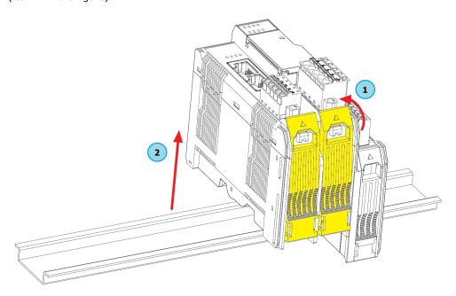
**NOTE** Disconnect all connections, including Ethernet, serial, and power cables, from the device before removing the device from the DIN rail.
