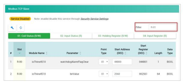
Point Type Category: Click 01: Coil Status (R/W), 02: Input Status (R), 03: Holding Register (R/W), or 04: Input Register (R) tab to see the registers under the specific point type.
