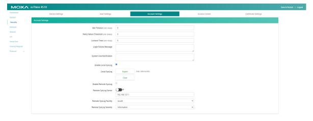
**Idle Timeout:** The timeout value when the user account is idle (unit: min(s), 0 to 1440 mins, default: 5 mins) Note: 0 for disabled.
