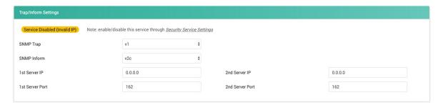
**SNMP Trap:** Select one of the SNMP version options (option: v1, v2c, or v3), through which the SNMP server can receive the SNMP Trap from the SNMP agent.
