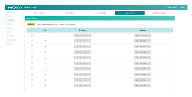
Enable access for a range of IP addresses by specifying the IP address and netmask, as follows:
