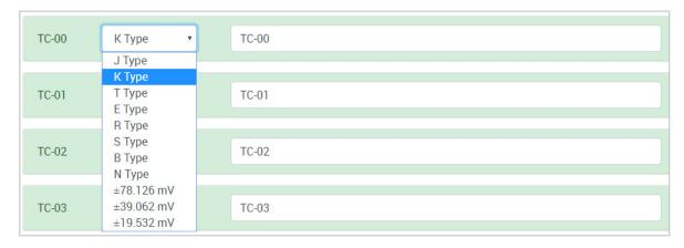
**Sensor Type Drop-Down List:** It lists all of the sensor types, which can be connected to this channel. Select the sensor type for each channel (option: J Type, K Type, T Type, E Type, R Type, S Type, B Type, N Type,  $\pm 19.532$  mV,  $\pm 39.062$  mV,  $\pm 78.126$  mV, or Disable).
