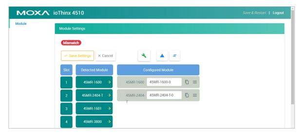
In edit mode, if any detected modules and configured modules do not match, then the configured modules will be highlighted as shown below.
