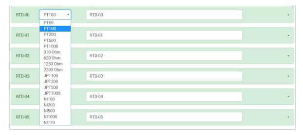
**Sensor Type Drop-Down List:** It lists all of the sensor types, which can be connected to this channel. Select the sensor type for each channel (option: PT50, PT100, PT200, PT500, PT1000, 310 ohms, 620 ohms, 1250 ohms, 2200 ohms, JPT100, JPT200, JPT500, JPT1000, NI100, NI200, NI500, NI1000, NI120, or Disable).
