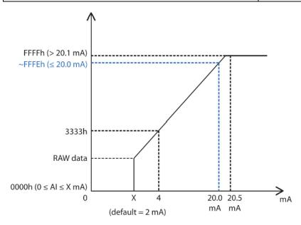
**1st Point Measured Value:** The 1<sup>st</sup> point value in the range of channel mode to be scaled to the **1st Point Scaled Value** (unit: mA, 4.000 to 20.000).
