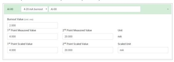
**Burnout Value (only for 4-20 mA burnout mode):** The 4-20 mA burnout mode is shown in the diagram below.
