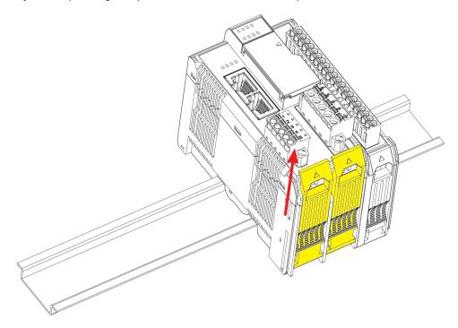
**Step 2:** Press the release tab (item 1 in the figure) and then remove the CPU module from the DIN rail (item 2 in the figure).
