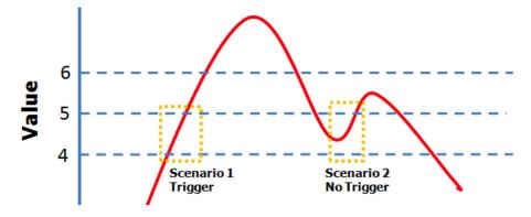
When Trigger = Less, Value = 5, and Hysteresis = 1, the SNMP trap will only be triggered if the analog signal fluctuates from 6 to 5, as depicted in Scenario 1 below. However, if we change the settings to Value = 5 and Hysteresis = 2, the SNMP trap will only be triggered if the analog signal fluctuates from 7 to 5.
