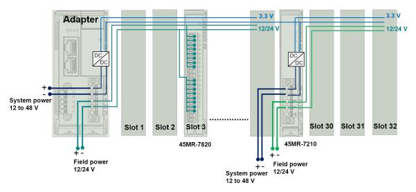
**NOTE** All I/O points have 3 kV VDC or 2 kVrms isolation with the system. We recommended using different power supplies to ensure that the system power and field power are isolated from each other.
