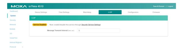
Message Transmit Interval: Set up interval time for message transmission via LLDP protocol.
