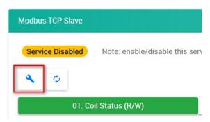
**Reload Configuration:** Click this button to reload the configuration settings of all Modbus registers.
