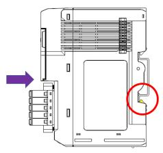
**INFORMATION** When the I/O module is inserted into the correct position, the connection between the internal bus and the previous module is established.
