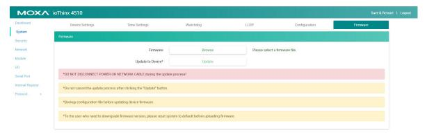
**NOTE** When the device is updating, do not turn the power off as it might corrupt the device.
