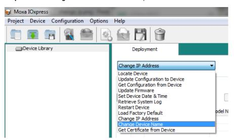
**Step 2:** Select the device(s), change the device name, type the **username** and **password**, and then click **Submit**. IOxpress will start to execute the task on the selected devices. A message indicating success will appear in the **Result** column if the process was completed successfully.
