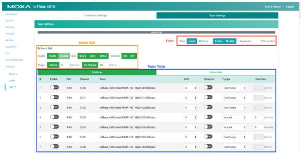
**Filter:** The ioThinx 4510 has a filter function in the top right corner of the subscribe page that allows users to find topics more easily. Click the **Value/Attribute/Enable/Disable** buttons and then type a keyword to find a topic within several seconds. The number of filtered topics will be shown as well.
