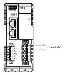
The amount of system current required to support an expansion module is 1 A. If more modules and more power consumption is needed, an additional power module (45MR-7210) is required. Below is an example:
