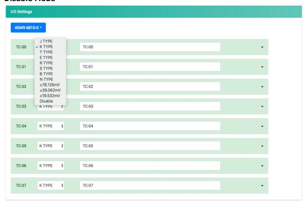
The TC channel can be disabled. You may only disable channels one-by-one. When a channel has been disabled, the sample rate of the remaining channels will be increased automatically.
