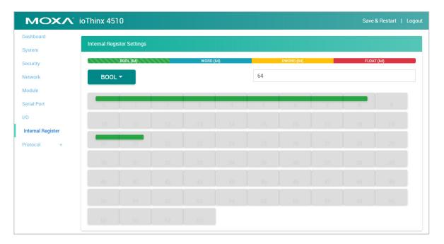
IR Type Drop-Down List: It lists all of the IR types. Select the IR type to modify or view its settings.
