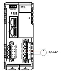
**NOTE** The 12/24 VDC field power supply can be connected directly to 45MR modules. If more connection points are needed, purchase 45MR-7820 (8 x FP+ and 8 x FP-) modules.
