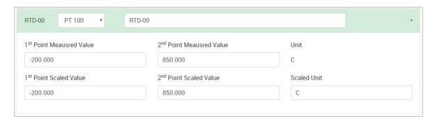
**1**<sup>st</sup> **Point Measured Value:** The 1<sup>st</sup> point value in the range of channel mode to be scaled to the **1st Point Scaled Value** (acceptable input value depends on the type of sensor).
