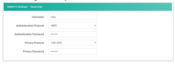
**Username:** Type the username for SNMP v3 settings (min. length = 1; max length = 30; A to Z, a to z, 0 to 9, symbols, spaces and  $.()[]{}/"@;:$  symbols are not allowed, default = "v3ro").
