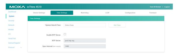
System Date & Time: Select the date for the device. Click Set Time to set the time of the device.
