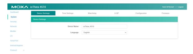
**Device Name:** Set the name of this device (max length = 16, '.' is not allowed).
