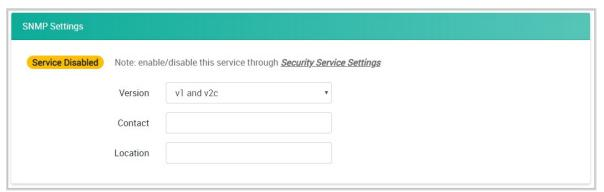
**Version:** Select one of the SNMP version options (option: v1 and v2c, v3 only, or v1 and v2c and v3), through which the SNMP Manager can access the SNMP agent of the device.
