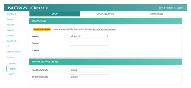
The ioThinx 4510 Series supports SNMP, SNMP Trap, and SNMP Inform. After configuring these settings, please download the mib file from Moxa's website. For detailed information on the structure of the mib file, please refer to the **SNMP** chapter.
