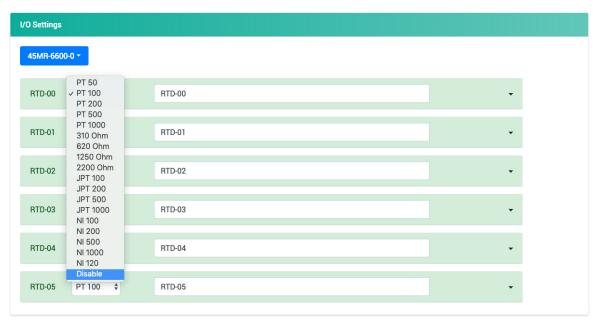
The RTD channel can be disabled. You may only disable channels one-by-one. When a channel has been disabled, the sample rate of the remaining channels will be increased automatically.
