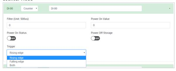
Filter: Software filtering is used to avoid switch bounces (unit: 500µs, 0 to 65535).
