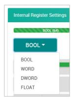
**IR Quantity:** Apply a number to adjust the quantity of the selected IR type. The total available IR quantity is 256.
