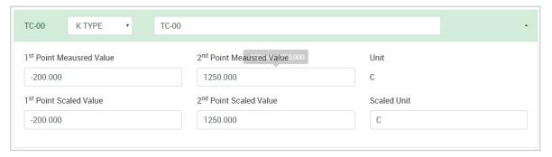
**1st Point Measured Value:** The 1<sup>st</sup> point value in the range of the channel mode to be scaled to the **1st Point Scaled Value** (acceptable input value depends on the type of sensor).
