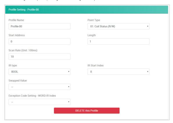
**Profile Name:** Name the profile of the Modbus device (max. length = 16; "." character is not allowed).
