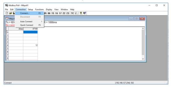
2. Enter the IP address of the device (default IP: 192.168.127.254).
