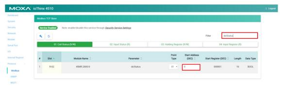
**NOTE** You can also manually modify the addresses if needed. To do so, click **Save & Restart** in the top right of the page after changing the **Start Address**.
