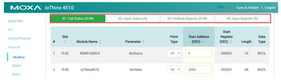
2. Type the text "doStatus" in the filter to find the **Start Address** of the DO channel.
