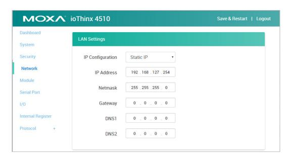
**IP Configuration:** Configure the following settings if **Static IP** is selected. If **DHCP** is selected, the following settings are not allowed (option: Static IP or DHCP).
