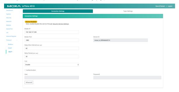
The ioThinx 4510 supports generic MQTT, and after configuring it, the ioThinx 4510 will connect the MQTT broker automatically. For detailed information about topics and payloads, refer to the MQTT section in Chapter 4.
