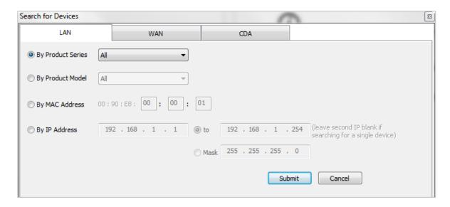
**NOTE** If the devices cannot be found, check the network setting of the devices.
