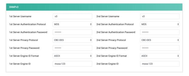
**Username:** Type the username for the SNMP v3 settings (min. length = 1; max length = 30; A to Z, a to z, 0 to 9, symbols, spaces and  $.()[]{}/"@;:$  symbols are not allowed, default = "v3").
