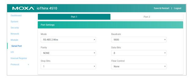
**Mode:** The standard of the serial device connected to this port (option: RS-232, RS-422, or RS-485 2-Wire).
