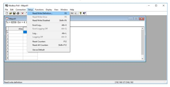
2. Select the **function** code **05 Write Single Coil** and then enter **0**, the start **Address** of the DO channel.
