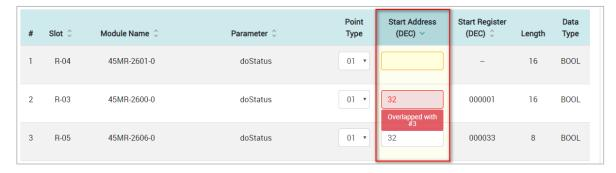
**Sort:** The default-sorted column is the **Slot** from the lowest to highest slot number. Click the green arrow to change the sorting method. Click the gray arrows on the other columns to sort that specific column.
