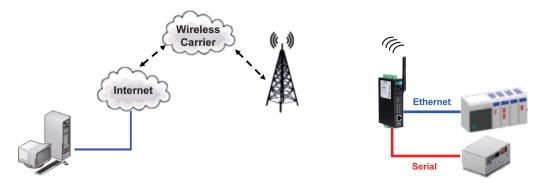
The OnCell G3150A-LTE enables traditional serial (RS-232/422/485) devices for transmitting data over the cellular network. The IP gateway is a computer equipped with a CPU and TCP/IP protocols that can bi-directionally translate data between the serial and IP formats. With the OnCell G3150A-LTE, your computer will be able to access, manage, and configure remote facilities and equipment over the cellular network from anywhere in the world.
