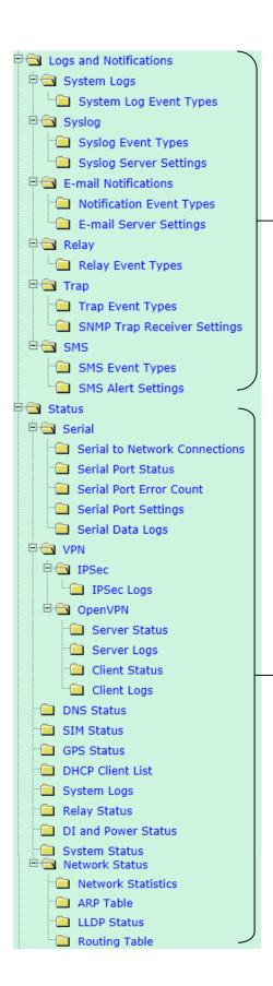
Application-oriented device management functions to set up events, traps, and responses via relay warning, email, and SNMP notification.
