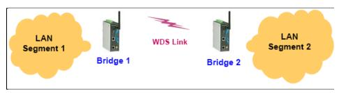
It is a good idea to plan your wireless network by drawing a diagram so that you know how each AWK-3121 is connected to other peer APs or wireless bridges by WDS, and how bridges are connected to other peer bridges by WDS. See the following figure for an example of a network-planning diagram.
