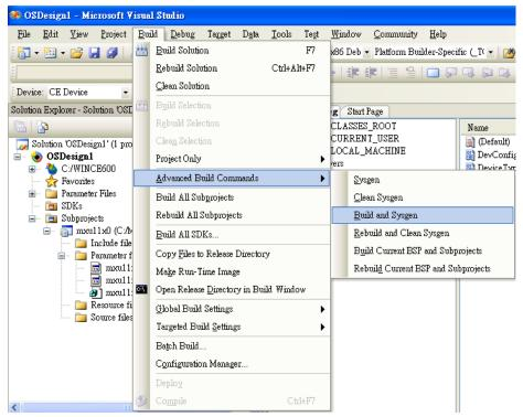
8. After building sysgen, select "Build" and "Make Run-Time I mage" to create the WinCE OS image. Finally, copy your image file to the target host.
