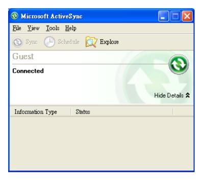
3. Click on the "Explore" button in the ActiveSync window and then copy the UP1100\_COM\_v1.0\_Setup.CAB (For WinCE 6.0) or UP1100\_COM\_v1.1\_Setup.CAB (For WinCE 5.0) file to the Mobile/Target Device.
