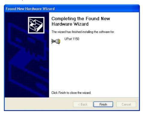
7. After Windows has completed installing the converter, it will automatically detect the new COM port. The **Found New Hardware** speech balloon will appear in the bottom right corner of the Windows desktop.
