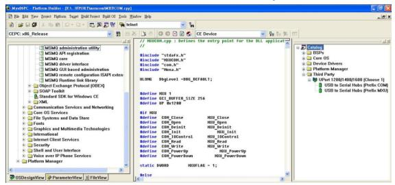
3. Right-click on the driver "USB to Serial Adapters (Prefix COM)" or "USB to Serial Adapters (Prefix MXU)" and then choose "Add to OS Design." After adding the driver, you should be able to find it in your workspace. At this point, you can start building your operating system and download it to a target.
