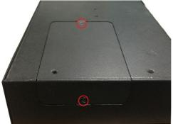
2. Remove the cover to access the SD-card slot and the mSATA socket.  $\ensuremath{\mathsf{mSATA}}$
