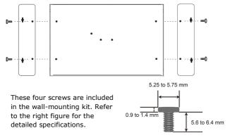
Next, use two screws per bracket to attach the UC-8410A to a wall or cabinet.
