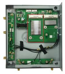
Install the cellular module onto the socket and fasten the two screws on the module.
