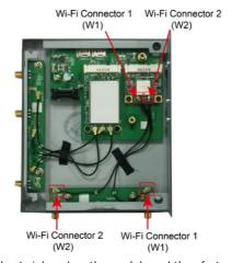
Install the heat sink pad on the module and then fasten two silver screws.
