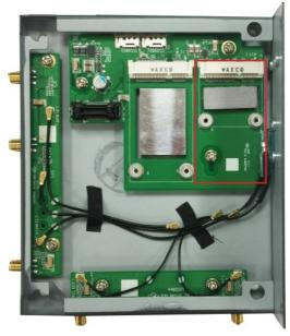
2. Remove the two silver screws on the socket.
