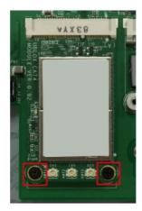
Connect the antenna cables to the antenna connectors.
