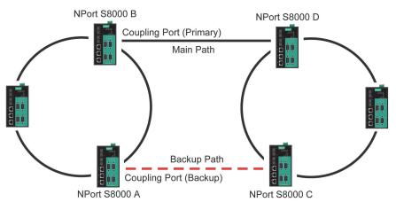
Note that the ring coupling settings for a "Turbo Ring V2" ring are different from a "Turbo Ring" ring. For Turbo Ring V2, Ring Coupling is enabled by configuring the "Coupling Port (Primary)" on Switch B, and the "Coupling Port (Backup)" on Switch A only. You do not need to set up a coupling control port, so that a "Turbo Ring V2" ring does not use a coupling control line.
