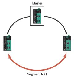
If there are 2N+1 NPort S8000 (an odd number) in the "Turbo Ring" ring, with NPort S8000 and segments labeled counterclockwise, then segment N+1 will serve as the backup path.
