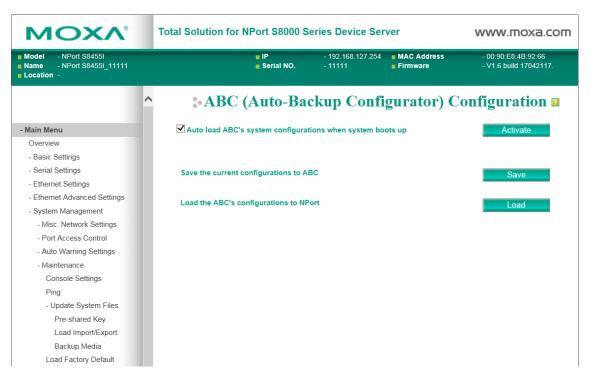
You can use Moxa's Automatic Backup Configurator (ABC-01) to save and load the NPort S8000's configurations through NPort S8000's RS-232 console port. You may find more details about ABC-01 at: <a href="http://www.moxa.com/product/Automatic Backup Configurator ABC-01.htm">http://www.moxa.com/product/Automatic Backup Configurator ABC-01</a>.
