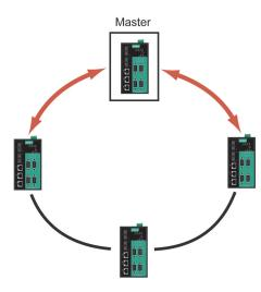
For a "Turbo Ring V2" ring, the backup segment is the segment connected to the second redundant port on the master.
