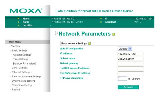
You must assign a valid IP address to the NPort S8000 before it will work in your network environment. Your network system administrator should provide you with an IP address and related settings for your network. The IP address must be unique within the network (otherwise, the NPort S8000 will not have a valid connection to the network). First time users can refer to Chapter 3," Initial IP Address Configuration", for more information.
