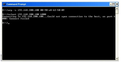
5. After the NPort S8000 reboots, its IP address will be assigned to the new address, and you can reconnect using Telnet to verify that the update was successful.
