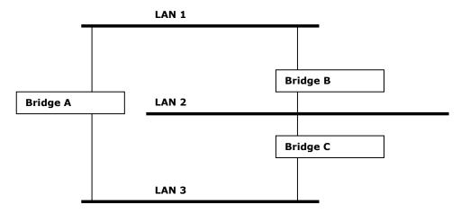
The figure below shows a network made up of three LANs separated by three bridges. Each segment uses at most two paths to communicate with the other segments. Since this configuration can give rise to loops, the network will overload if STP is NOT enabled.
