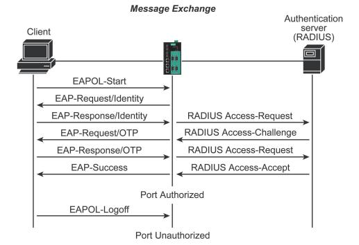
1. When the supplicant receives an "EAP Request/Identity" frame, it sends an "EAP Response/Identity" frame with its username back to the authenticator.
