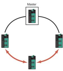
If there are 2N NPort S8000 (an even number) in the "Turbo Ring" ring, then the backup segment is one of the two segments connected to the (N+1)st NPort S8000 (i.e., the NPort S8000 unit directly opposite the master).
