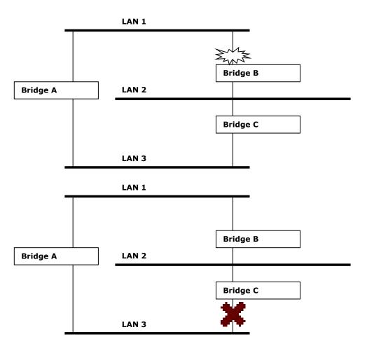
What happens if a link failure is detected? As shown in next figure, the STP process reconfigures the network so that traffic from LAN segment 2 flows through Bridge B.
