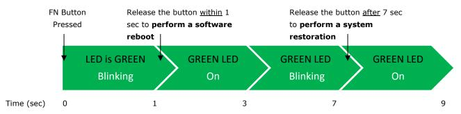
The mapping of the action on the FN button with the behavior of the SYS LED and the resulting system status is given below:
