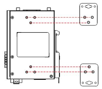
2. Use two screws to mount the UC-3100 on to a wall.
