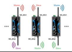
∆WLANs with same color must have identical RF type, SSID, and security settings.
