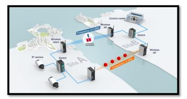
3. **Device Failover:** After covering the communication and frequency failures, in order to provide a singlepoint-of-failure free wireless network, AeroLink Protection also checks the device status. If the Active node has a power failure, the Backup nodes will automatically resume the wireless communication.
