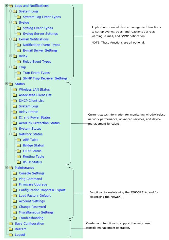
The management functions are categorized in a tree and shown in the left field of the web-based management console. You can efficiently locate the function you need with this guide.
