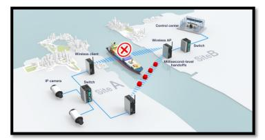
Frequency-Interference Failover: This concept is similar to the previous model. If the communication frequency experiences interference and data can no longer be transmitted over the Active frequency, it will resume the connection via another Backup frequency.
