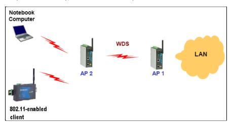
By using WDS, two or more LAN segments can be connected wirelessly. As illustrated in the figure below, a pair of wireless LAN-to-LAN bridges is used to connect two LAN segments. Since the AP is WDS-enabled, it can be used as a wireless bridge.
