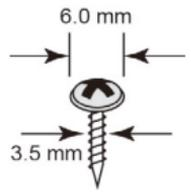
Do not screw the screws in all the way—leave a space of about 2 mm to allow room for sliding the wall mount panel between the wall and the screws.
