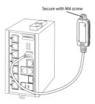
Avoid hanging the ABC-02 configurator from the switch without securing it onto the wall.
