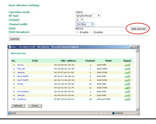
NOTE If the Gateway field in Basic Settings → Network Settings is empty, a warning message will appear, reminding you to set the default gateway when Client mode is enabled. You can ignore this message if you are only planning a local network and packets will not be sent outside the network.
