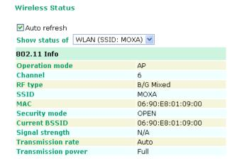
**NOTE** The **802.11 info** that is displayed may be different for different operation modes. For example, "Current BSSID" is not available in Client mode, and "Signal strength" is not available in AP mode.
