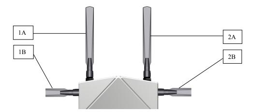
The AWK-6232 supports 802.11 a/b/g/n with 2x2 MIMO technology and dual RF redundancy. Antennas 1A and 1B are the MIMO antennas associated with RF1, and 2A and 2B are the MIMO antennas associated with RF2.
