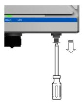
**STEP 2:** Using a pointed object, press and hold the reset button.
